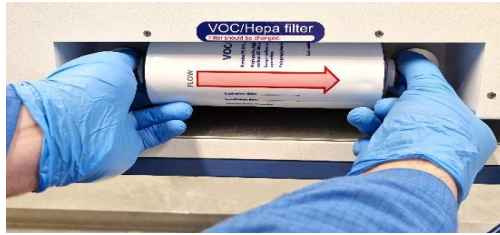
Figure 12.2 VOC/HEPA filter insertion and removal procedure
