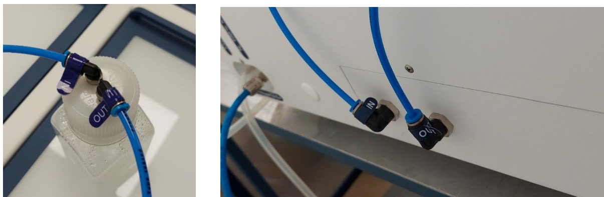
Figure 23.1 Tube connection on the humidification bottle and the MIRI® Humidity multiroom IVF incubator
